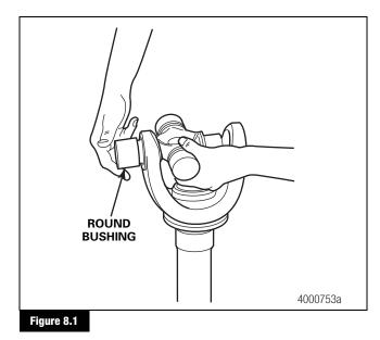
2. Press the first round bushing into the yoke slightly past the snap ring groove. Check that the bushing is aligned with the universal joint trunnion. Figure 8.2.
