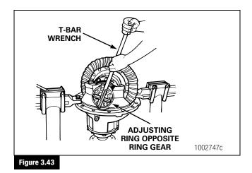
5. Remove the capscrews and washers that fasten the bearing caps to the differential carrier. Mark the bearing caps and the carrier to help you correctly assemble the caps into the carrier.
