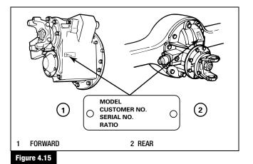
Compare the axle ratios shown on both tags. To operate correctly, the axle ratios for both axles must be within one percent of each other. To calculate the percentage difference between the axle ratios, refer to the equation in Table E.
