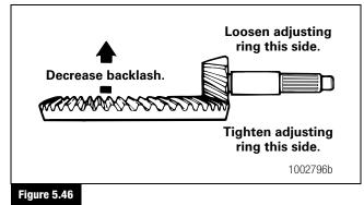
**NOTE:** When you adjust the backlash, only move the ring gear. Do not move the drive pinion.
