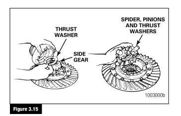
5. If the ring gear needs to be replaced, remove the bolts, nuts and washers, if equipped, that hold the gear to the flange case half.
