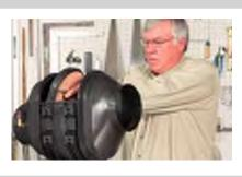
The safety filter should be replaced every three primary filter changes.
