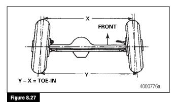
**NOTE:** Toe-in must be measured with the weight of the vehicle on the axle and the axle on a level floor. Use the following procedure.
