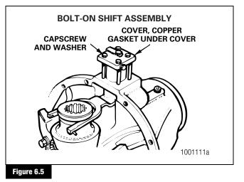
Remove the capscrews, cotter pins, roll pins or lock plates, if equipped, that hold the two bearing adjusting rings in position. Use a small drift and hammer to remove the pins. Each lock plate is held in position by two capscrews.
