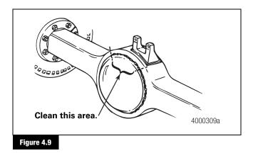
5. For suspension bracket welds, clean both lower and upper suspension brackets and the areas of the axle housing around each bracket. Use a wire brush and a cleaning solvent that will remove dirt and grease from these areas. Figure 4.10 and Figure 4.11.
