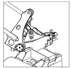
3. Move adapter toward "bucket close" position until outer end of adapter contacts bucket. Ensure proper alignment and continue to close until adapter contacts stops (1).
