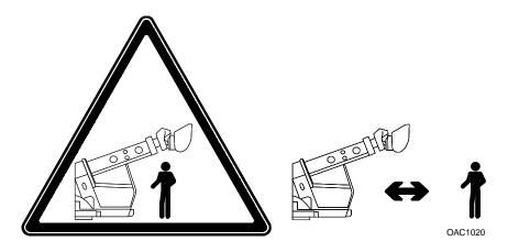
• Never permit anyone under boom, attachment or load. Rest boom or attachment on ground and stop engine before permitting anyone to work beneath boom or behind cradle.
