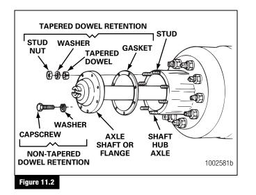
7. Install a cover over the open end of each hub where an axle shaft was removed. This will prevent dirt from entering the bearing cavity and loss of lubricant.
