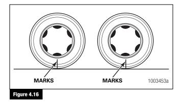
6. Turn the forward driveshaft in one direction by hand until the forward tire completes two rotations. Figure 4.17. The forward tire must rotate two times only. If the forward tire rotates more than or less than two rotations, the angle measurements you make in Step 7 will be inaccurate.
