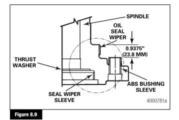
2. If disassembled, install the thrust washer and seal wiper sleeve into the spindle. Figure 8.10.
