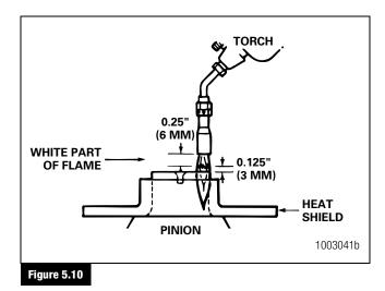
5. Remove the flame and the heat shield from the pinion. Let the pinion air cool for 10 minutes. Use a razor blade to remove the temperature indicating liquid.
