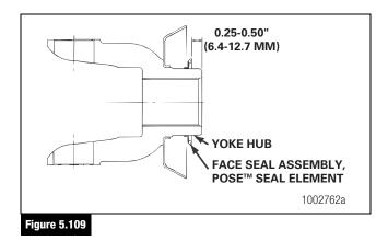
4. Before you install the yoke or flange onto the shaft, apply axle lubricant to the hub.
