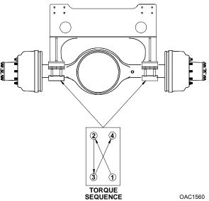
Torque bolts in a 4 stage, criss-cross pattern:
