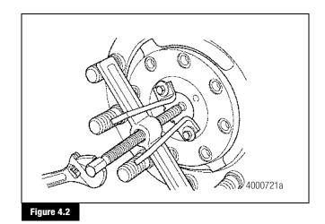
9. Remove the outer adjusting nut, lock ring and the inner adjusting nut from the spindle. Use the correct size wrench socket to remove the adjusting nut. Figure 4.3.
