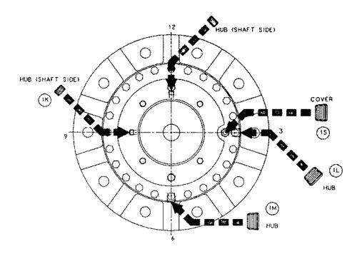
This figure shows the most common pipe plug timing for this series. Pipe plug timings may vary among units with different model numbers. Refer to an original assembly print for your particular unit to determine its correct pipe plug timing.
