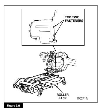
2. Remove all but the top two carrier-to-housing capscrews or stud nuts and washers. Figure 3.9.
