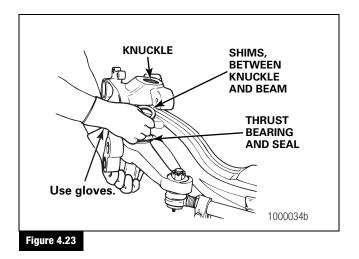
10. Remove the knuckle from the axle beam. Figure 4.24. Inspect the parts. Refer to Section 5.
