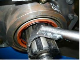
5. Remove the seal sleeve from the yoke (if applicable), taking care not to damage the yoke OD where the sleeve rides.
