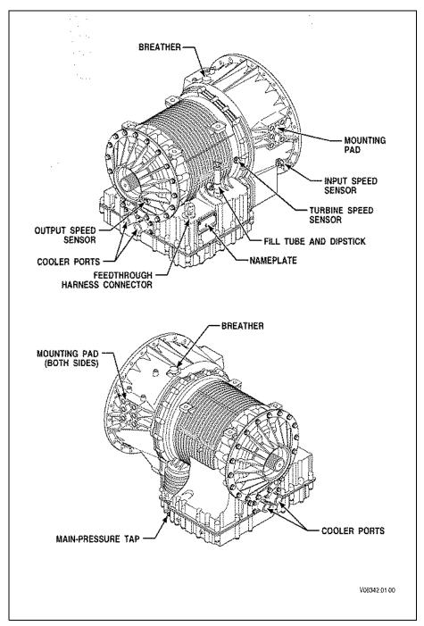
Figure 5–2. 4000 HS and 4500 HS (Allison 4<sup>th</sup> Generation Controls)
