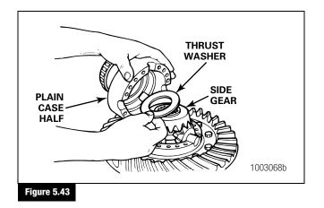
14. Place the plain half of the differential case over the flange half and gears. Rotate the plain half to align the match marks. Figure 5.43 and Figure 5.44.
