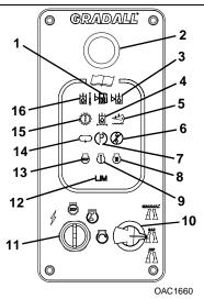
**Note:** When key is turned to the "RUN" position (see page 2-44 for details), the engine stop, check engine, and optional engine preheat displays illuminate for approximately two seconds and then go off. Depending on the temperature, the optional engine preheat light may continue to illuminate until the intake manifold warms to proper temperature.
