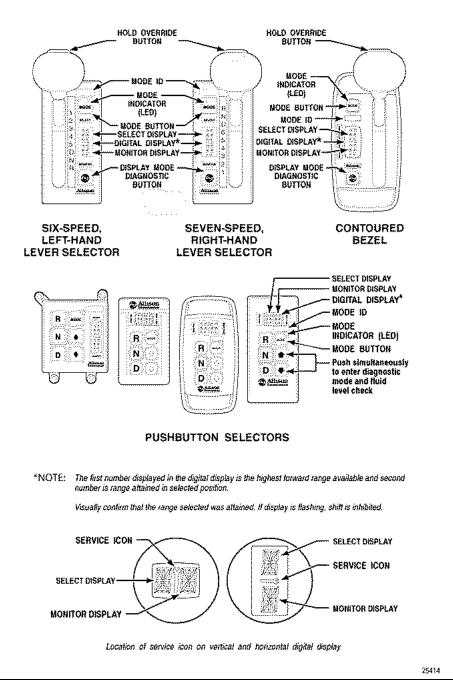
Figure 7–1. Typical Allison 4<sup>th</sup> Generation Prognostics Shift Selectors
