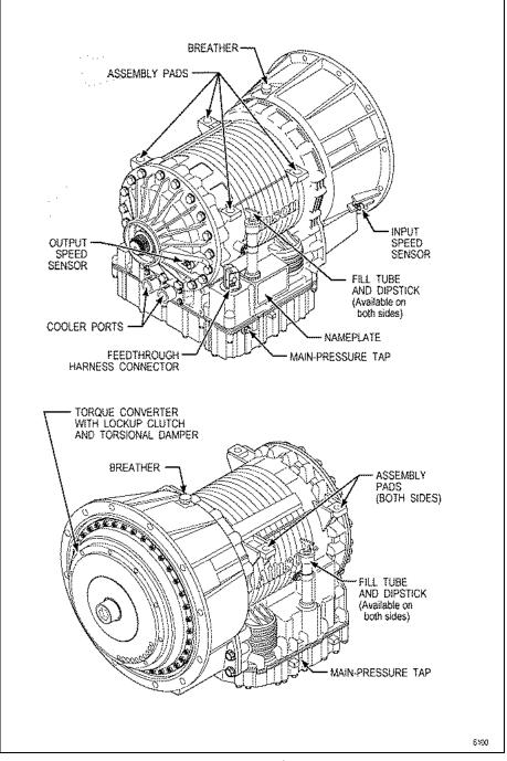
Figure 5–1. 3000 HS (Allison 4<sup>th</sup> Generation Controls)
