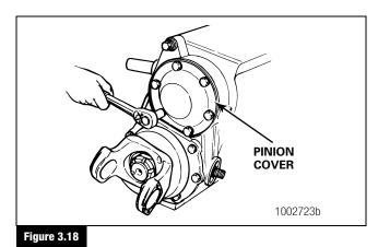
3. Use the correct tool to hold the input yoke or flange. Loosen, but do not remove, the drive pinion nut. Figure 3.19.
