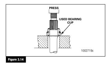
3. Press the thru-shaft through the bearing cones. Discard the bearing cones.
