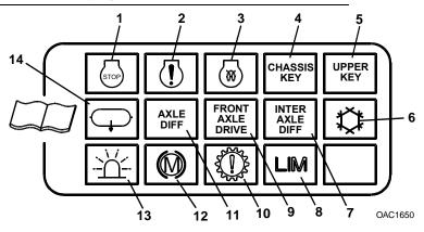
**Note:** When ignition is turned to the "RUN" position (see page 2-27 for details), the engine stop, check engine, and optional engine preheat displays illuminate for approximately two seconds and then go off. At lower temperatures, the optional engine preheat light may continue to illuminate until the intake manifold warms to proper temperature.
