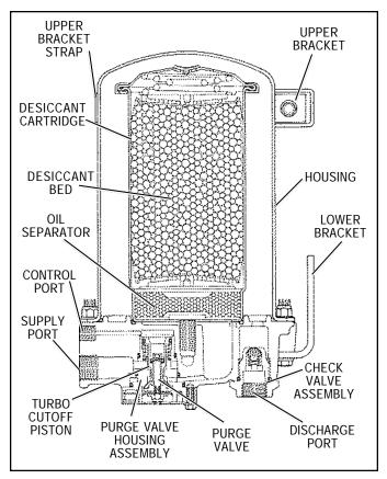
FIGURE 5 - AD-9<sup>™</sup> AIR DRYER SECTIONAL VIEW
