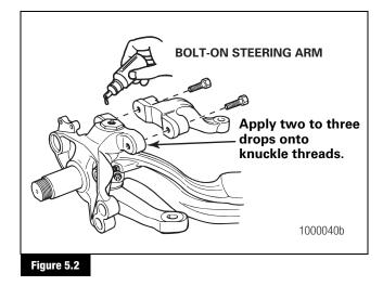
3. Tighten the fasteners to the required torque value for that size fastener. Refer to Section 10.
