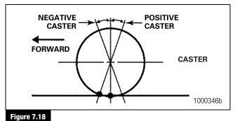
Always use an alignment machine to check the caster angle. When checking caster, refer to the alignment equipment manufacturer's procedures.
