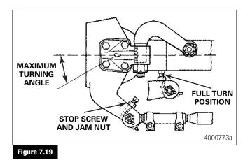
2. Lock the steering stop in position with the jam nut tightened to 180-230 lb-ft (244-312 N•m). ●
