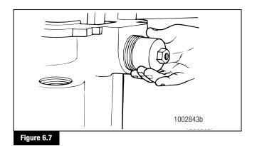
5. Place the shift cylinder and piston assembly in a vise that has brass covers over the jaws. Remove the piston and O-ring from inside the cylinder. Use a narrow drift through the hole in the top of the cylinder to push out the piston. It may be necessary to use a mallet to tap out the piston. Figure 6.8.
