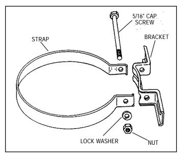
FIGURE 10 - UPPER MOUNTING BRACKET AND STRAP
