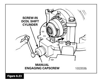
11. Turn the manual adjusting capscrew to the right until the head is approximately 0.25-inch (6 mm) from the cylinder cover. Do not turn the capscrew beyond its normal stop. The capscrew is now in the service position and the main differential lock is completely engaged.
