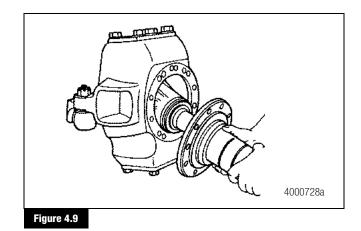
**NOTE:** The felt seal and retainer are not included with the greaseable drive flange design.
