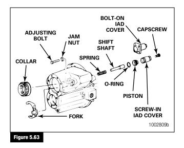
2. Place the spring and the shift fork into position in the carrier. The spring must touch the screw side of the carrier. The boss on the fork must be toward the adjusting bolt.
