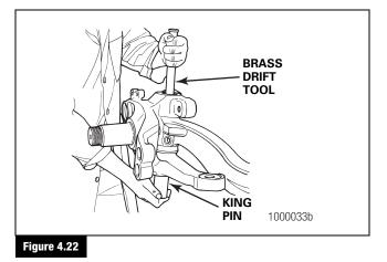
8. If the king pin is hard to remove, use a hydraulic king pin remover. Refer to Section 11. To obtain this tool, refer to the Service Notes page on the front inside cover of this manual.
