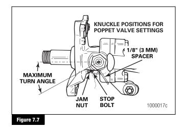
**NOTE:** If the steering system is out-of-adjustment, inspect the steering arm for damage. Use a magnetic particle or liquid dye penetrant inspection procedure to inspect the steering arm. Pay particular attention to the bend, the taper and the area near the ball stud. Refer to the vehicle manufacturer's manual for additional inspection procedures.
