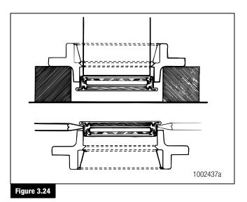
If the pinion bearings need to be replaced, remove the inner and outer bearing cups from the inside of the cage.
