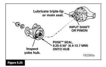
4. Slide the yoke over the input shaft pinion. Align the yoke splines with the shaft splines.
