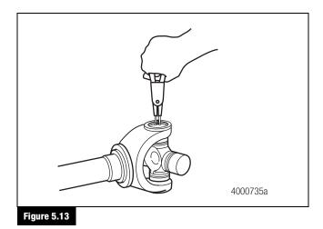
2. If necessary, use a brass drift and lightly tap the center of the bushing to assist in snap ring removal. Figure 5.14.
