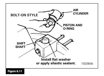
Install the O-ring into its groove on the piston. Lubricate the O-ring with axle lubricant. Install the piston into the air cylinder. Figure 6.11.  Install the cylinder into the housing bore. Verify that the pilot journal on the piston is against its bore on the shift shaft. Figure 6.12.
