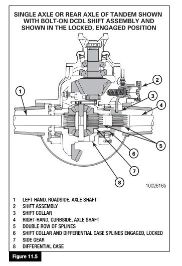
14. Lock or engage the main differential using the manual engaging method.
