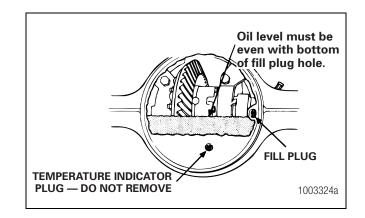
5. Install the fill plug. Tighten the plug to 35-50 lb-ft (48-67 N•m).
