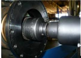
4. Remove the existing seal with a seal puller, taking care not to damage the seal bore
