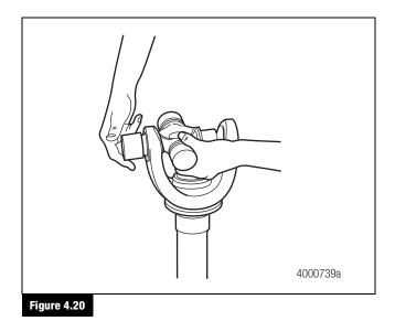
7. Turn over the universal joint. Repeat the procedure for the opposite side of the universal joint. Figure 4.21.
