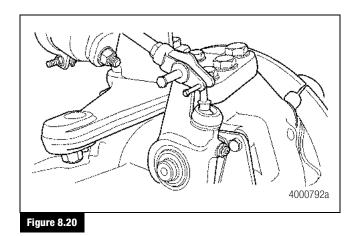
The distance from the back of the brake air chamber to the center of the clevis pin is the brake slack adjuster position (BSAP). Adjust slack adjuster position to obtain the correct specification in Table F.
