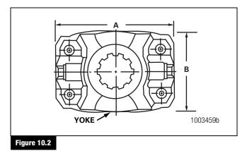
Calculate dimensions C and D of the yoke bar by adding 0.125-0.250-inch to dimensions A and B of the yoke. Figure 10.3.
