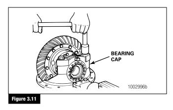
7. Remove the bearing caps and bearing adjusting rings from the carrier. Figure 3.12.
