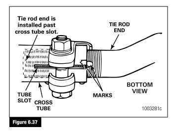
If you are installing new tie rod ends, thread the tie rod ends to the approximate original depth inside the cross tube. Figure 6.38.
