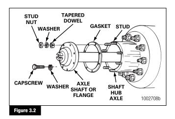
5. Install a cover over the open end of each axle assembly hub where an axle shaft was removed.
