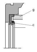
If the shaft is deeply grooved, insert a shim behind the shaft seal.
