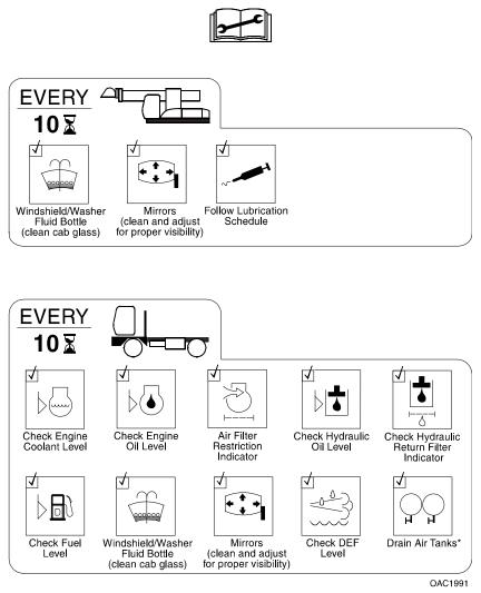
\* Drain air tanks daily. To prevent possible damage to emission controls components, wait a **minimum** of 10 minutes after shutting off engine before draining air tanks.
