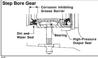
Maintain grease pack behind the output shaft dirt and water seal as a general maintenance procedure at least twice a year, in the Spring and Fall. Grease fitting is provided in housing trunnion. Use only NLGI grade 2 multipurpose chassis lube, and use only a hand operated grease gun on fitting. Add grease until it begins to extrude past the sector shaft dirt and water seal.
