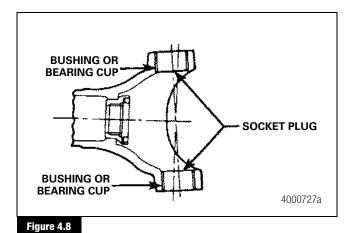
9. If necessary, remove the bushings or bearing cups and the socket plugs from the upper and lower sockets in the housing.
