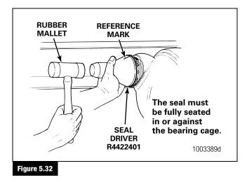
5. Visually inspect the seal to verify that it is seated correctly.
