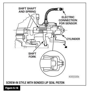
1. Install the shift fork into the shift of the carrier. The "L" shape of the fork and the bore for the shift shaft must face out toward the cylinder bore in the side of the carrier. Figure 6.17.
