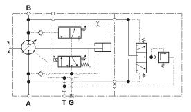
EP1 and EP2 Control with Flushing Valve
