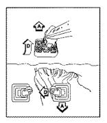
11. Move left joystick to left **(G)** or right **(H)** to align boom for next cut. Repeat steps 3 through 11.
