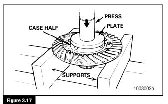
8. If the differential bearings need to be replaced, use a bearing puller or press to remove the bearing cones from the case halves. Figure 3.18.
