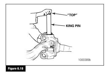
12. Rotate the king pin so that the two draw key slots of the pin correctly align with the draw key slots in the knuckle.
