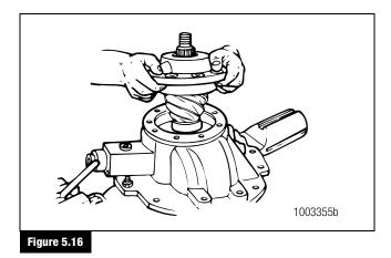
3. Install the bearing cage-to-carrier capscrews. Washers are not required at this time. Hand-tighten the capscrews.
