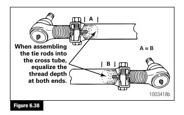
Both tie rod ends must be installed into the cross tube deeper than the end of the cross tube slot. Figure 6.37.
