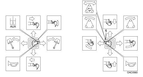
Joystick controls standard SAE control pattern. If tilt speed has been reduced for conditions, speed can be temporarily increased by depressing fast tilt button (1).
