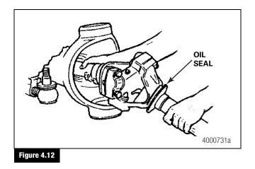
2. Remove the oil seal from the outer drive shaft. Discard the seal. Figure 4.12.
