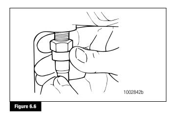
4. Remove the shift cylinder and piston assembly from the carrier by turning it to the left. Figure 6.7.
