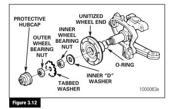
Install the tabbed washer and outer wheel bearing nut onto the spindle. Tighten the outer wheel bearing nut to 200-300 lb-ft (271-476 N•m). ●
