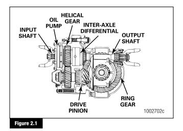
The Meritor 140, 145 and 160 forward tandem axles use a single-reduction, thru-drive carrier. The drive gearing is a two-helical gear train and a hypoid ring gear and pinion. Bevel gears are used in the main differential and the inter-axle differential. Figure 2.1 and Figure 2.2.
