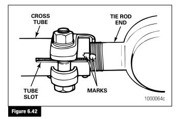
2. Install the nuts and the bolts into the clamps. Tighten to the specified torque. Refer to Section 10.
