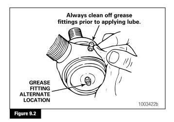
4. Attach either a hand or air pressure grease gun to the grease fitting. Figure 9.3. If using air pressure, do not exceed 150 psi (1035 kPa).
