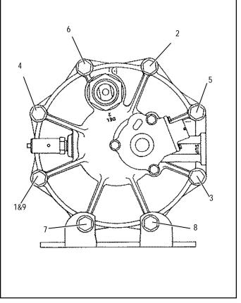
FIGURE 8 - END COVER TO HOUSING TORQUE PATTERN
