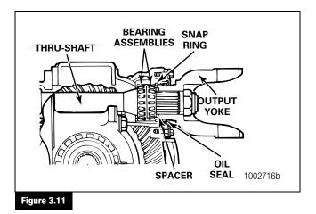
**NOTE:** If you replace either the bearing cup or the cone, replace both parts in a fully-matched set from the same manufacturer.
