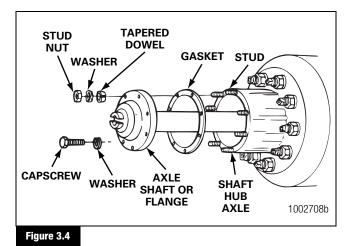
5. Install a cover over the open end of each axle assembly hub where an axle shaft was removed.
