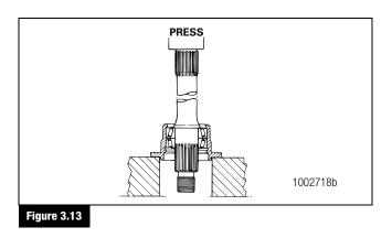
5. Use a press or a bearing puller to remove the bearing cones from the thru-shaft. Refer to the procedure in this section.
