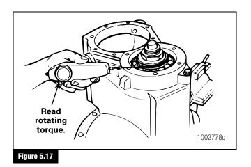
4. Measure the outer diameter of the washer under the drive pinion. Divide the outer diameter of the washer by two (2) to get the radius of the washer. Multiply the radius of the washer by the reading on the spring scale to get the preload on the pinion bearings.
