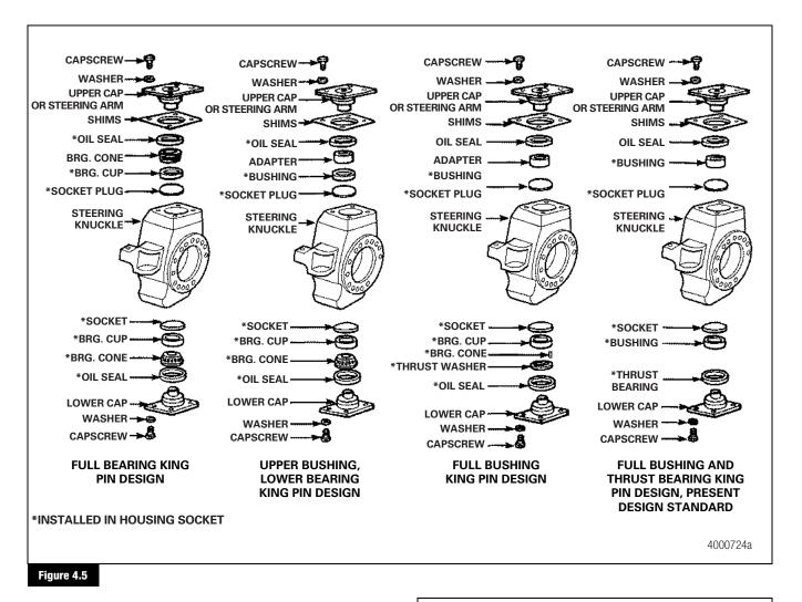
On axles above 16,000 lb (7258 kg) GAWR, the steering knuckle must be disassembled before the steering universal joint can be removed. On 16,000 lb (7258 kg) axles with the 850 joint, FDS-1600, the knuckle does not have to be disassembled.
