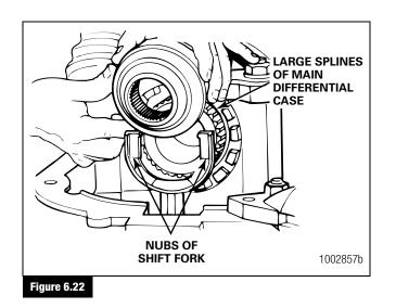
Engage the splines of the collar with the splines of the differential case. Insert the manual engaging capscrew through the top of the shift cylinder to move the shift collar toward the differential case. Rotate the collar as necessary to align the splines. Figure 6.23.
