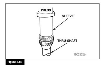
3. Use a press and sleeve to install the inner bearing cup into the cage. Place the thru-shaft and bearing assembly into the cage.
