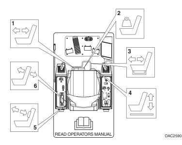
Prior to starting engine adjust seat for position and comfort.
