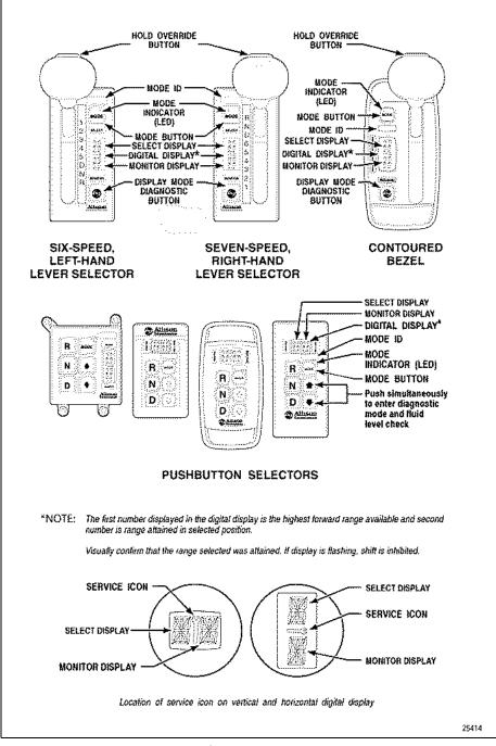
Figure 4–1. Typical Allison 4<sup>th</sup> Generation Prognostics Shift Selectors
