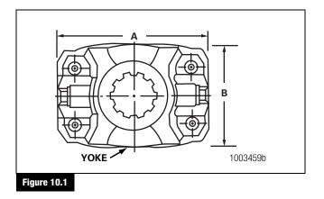
Calculate dimensions C and D of the yoke bar by adding 0.125-0.250-inch to dimensions A and B of the yoke. Figure 10.2.
