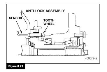
2. With the sensor in place, feed any excess cable back through the grommet on the knuckle. Do not affect the position of the sensor or allow excess cable to contact the drive shaft.
