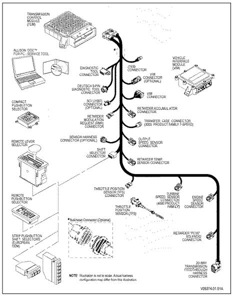
Figure 8–1. Typical Allison 4<sup>th</sup> Generation Controls Components
