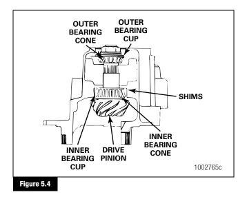
The preload of the bearings on the drive pinion is controlled by a spacer between the outer bearing cone and the helical driven gear.
