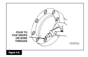
3. Tighten the fasteners to the required torque value for that size fastener. There is no drying time required for Meritor liquid adhesive 2297-C-7049, Loctite<sup>®</sup> 638 or 680 liquid adhesive or equivalent.
