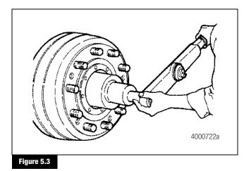
10. Remove the hub, drum and wheel assembly, if still mounted, straight off the spindle. If necessary, hit the inside of the wheel with a mallet to loosen it. Prevent the outer bearing cone from falling when you remove the hub.
