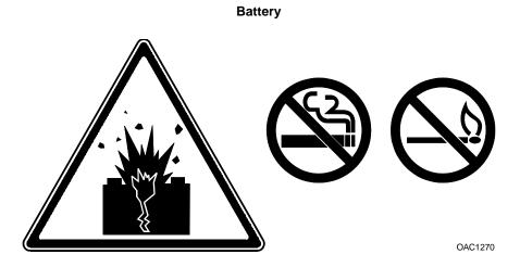
• Keep sparks, flames and lighted material away from batteries. Explosive gases could cause death or serious injury.
