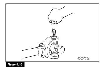
2. If necessary, use a brass drift and lightly tap the center of the bushing to assist in snap ring removal. Figure 4.17.
