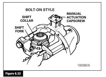
15. While the shift collar is still in the locked position, place the sensor switch, with the locknut loosely attached, into its hole.
