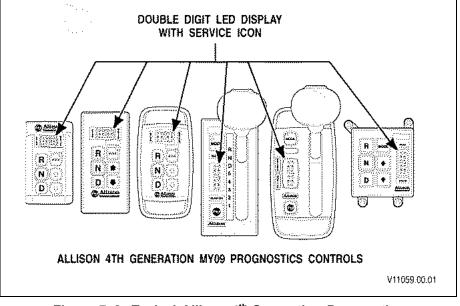
Figure 7–2. Typical Allison 4<sup>th</sup> Generation Prognostics Controls Shift Selectors with SELECT, MONITOR Digital Displays and Trans Service Indicator
