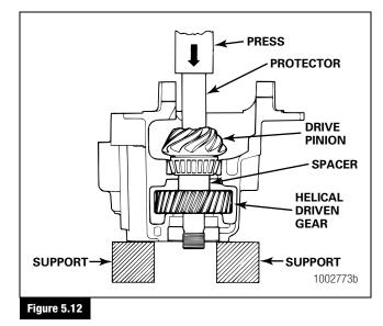
5. Install the drive pinion into the helical driven gear. Verify that the splines on the pinion engage the splines inside the gear. Figure 5.12.
