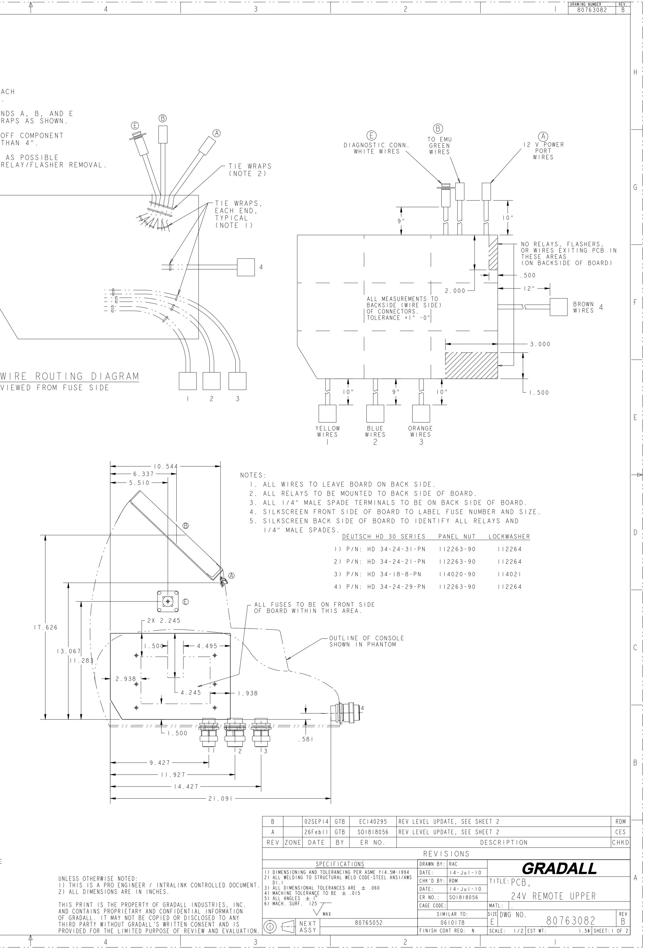
CONSOLE FLANGE CONTACT AREA. ALL PROTRUDING COMPONENTS AND TERMINAL ENDS ARE TO BE TRIMMED AS CLOSE AS POSSIBLE TO CIRCUIT BOARD IN THIS AREA (FUSE SIDE)
