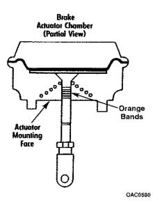
**Note:** Brake actuator chamber is shown with digging brake applied and with brake worn to a point just before automatic adjustment. If orange band is visible, notify maintenance personnel for adjustment or repair.
