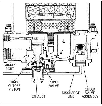
FIGURE 4 - AD-9<sup>™</sup> AIR DRYER TURBO CUTOFF
