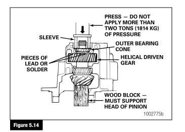
13. Release the pressure and remove the wood block from under the head of the drive pinion.
