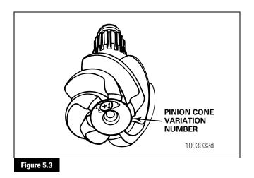
3. If you can't find the PC number or it's unreadable, install a new shim pack of the same thickness that you measured in Step 1.
