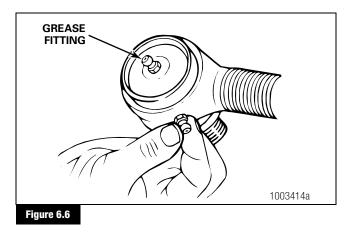
4. Tighten all grease fittings to the correct torque. Do not overtighten, which can damage the threads. Refer to Section 10.
