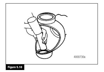
17. Clean all grease and dirt from the bores before reassembly.
