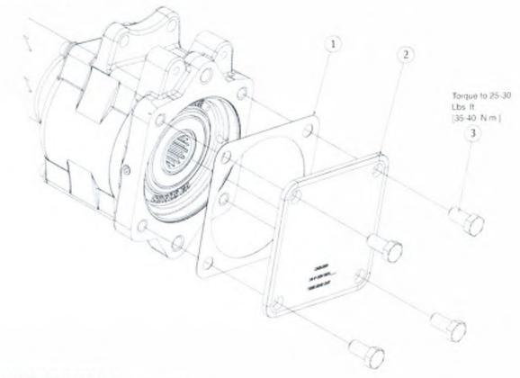
KITS: 329654X "XS", "CS" Oulput 329658X "XK", "AF", "AZ", "CK", "CF", "CZ" Output 329659X "XY", "CY" Output 329722X "DA" Output
