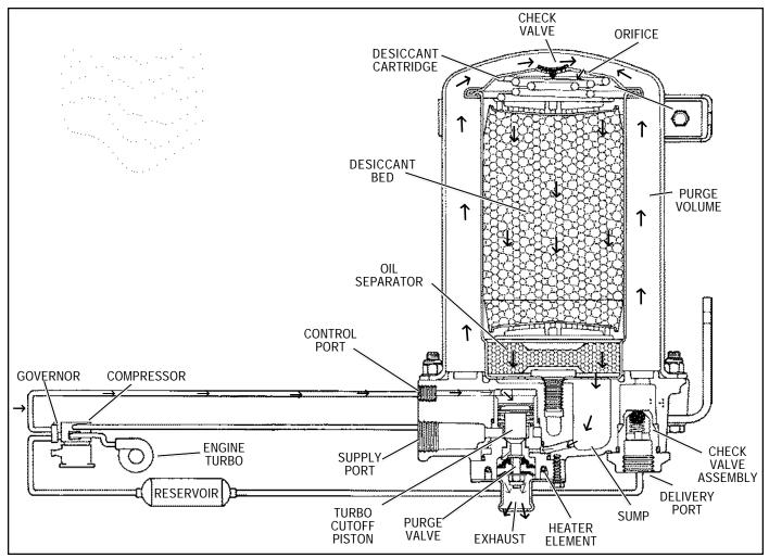
FIGURE 3 - AD-9™ AIR DRYER PURGE CYCLE
