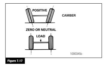
A small amount of positive camber is built into the knuckle, because camber changes with load. This results in a zero camber angle when the vehicle is operated at normal load.
