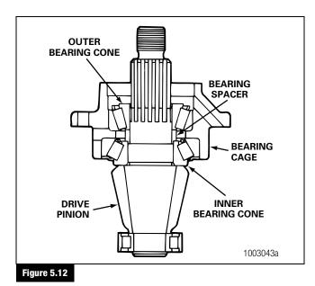
Install the outer bearing cone onto the pinion shaft against the spacer. Do not install the pinion seal into the bearing cage. Figure 5.12.
